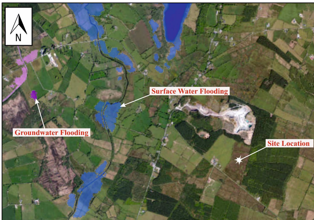
Plate 4. Extract from GSI Winter Surface Water Flooding Map 2015/16 with GSI's maximum historic groundwater flooding included.
